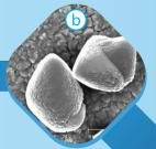
SEM micrographs of calcite deposits on surfaces obtained at room temperature from non-magnetized water (a) and magnetized with PURAK (b)
